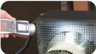
Stroboscope on: rotations visible
