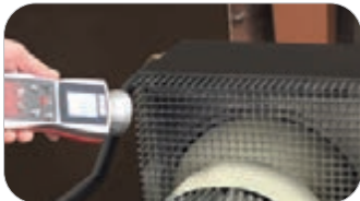
Stroboscope off: rotations not visible
