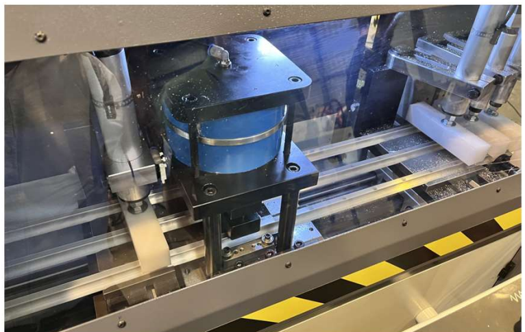
GAA-350 automatic cutting and punching Machine for three profiles at the same time with very high production rate for solar panels clips
