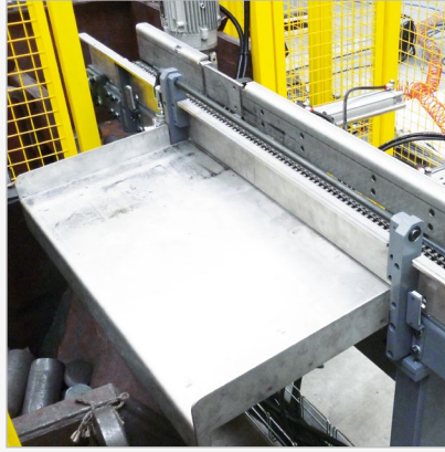
Output sorting table with chute - possibility of simultaneous withdrawal of several pieces - robust design for heavy pieces - adjustable angle of inclination
