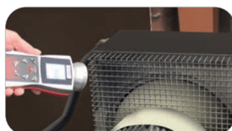
Stroboscope off: rotations not visible
